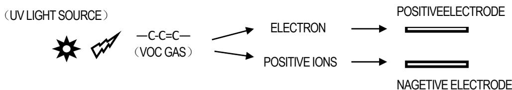
When UV light is applied to VOC molecules, the VOC will be ionized to produce positively charged ions and electrons. If a pair of collecting electrodes is placed in the ionized region, the electrons will flow to the positive electrode and the positive ions to the negative electrode to create an electric current, which is the signal output of the PID and proportional to the VOC concentration.
